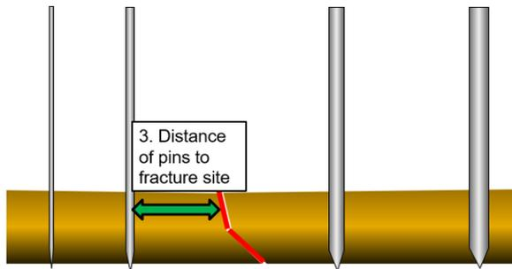
4. Through **larger distances between the pins** in a fragment, the holding strength increases.
