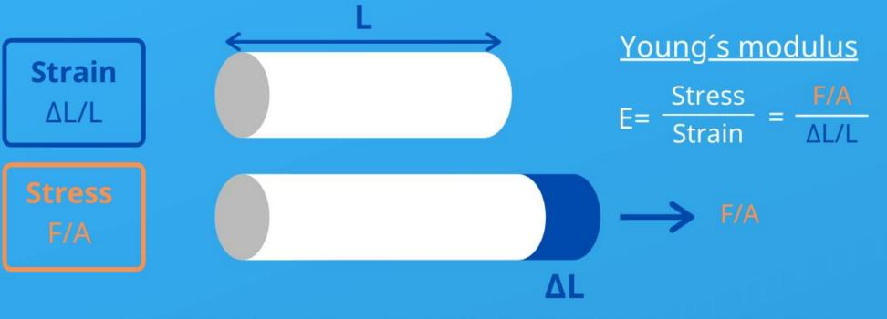
Young's modulus can be used to predict the elongation or compression of an object as long as the stress is less than the yield strength of the material.
