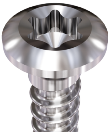
Fig 5 Star drive recess allows improved torque transmission and an increased resistance to stripping.
