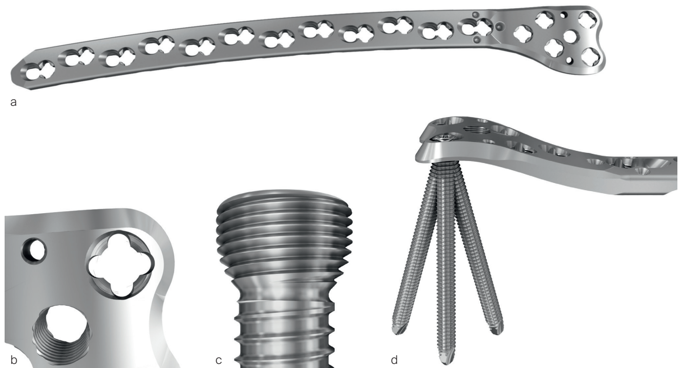
Fig 1a–d A 4.5 mm VA-LCP Condylar Plate in stainless steel with VA combi-holes in the plate shaft (a). Four columns of threads in the VA locking hole (b) provide four points of threaded locking between the VA-LCP plate and the VA locking screw (c). Screws can be angled within a 30° cone around the central axis of the plate hole (d).
