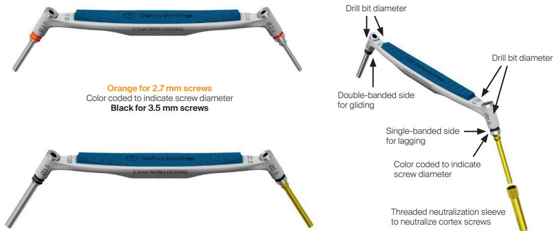
Fig 3 The 2.7 mm and 3.5 mm Non-Locking Drill Guides (left) and their design features as exemplified on the 3.5 mm instrument (right). Instead of using the spring-loaded feature of the former drill guide to drill a hole for a neutralized cortex screw, a Neutral Sleeve Adapter can be mounted to the lag screw side of the instrument to achieve the neutral position.
