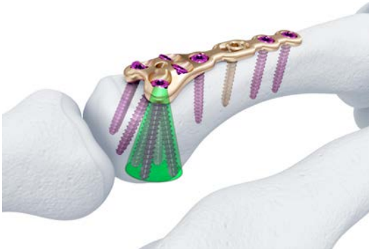
Fig 2 The variable angle locking hole provides freedom of screw placement within a 30° cone.
