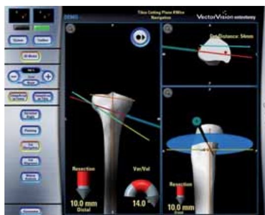
Fig 7 Actual and planned cutting tool position.
