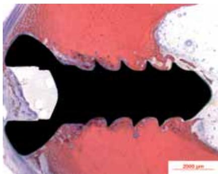
**Fig 2** Polished titanium cortex screw after 12 weeks within a sheep tibia showing good bony growth between the threads, but with less direct bone contact compared to the standard microrough titanium screws. It was shown that polishing also reduced the removal torque.
