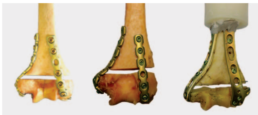
Implants tested: conventional reconstruction plates, LCP reconstruction plates and distal humerus plates (from left) applied to human distal humerus specimens in 90° configuration.
