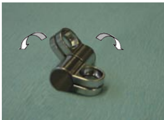
Fig. 1: The rod with the axial laser line and two symmetric clamps that can be flipped to either side of the rod (arrows).
