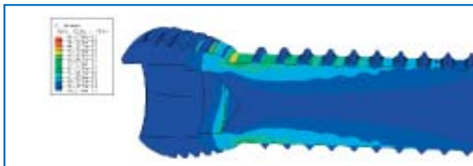
Fig 1: Stress distribution in a locked screw with HEX drive under bending load.
