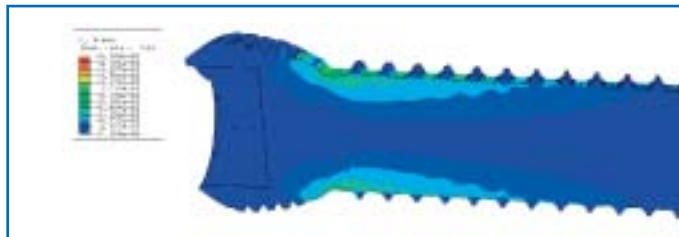
Fig 2: Stress distribution in a locked screw with Stardrive® under bending load.
