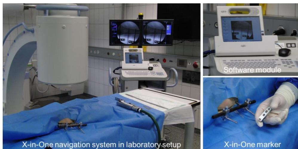
Figure 10.5.3: Navigation tool for assisting rotational osteotomies in a laboratory setup, containing the software module implemented on a tablet computer (upper right) and the special designed markers (lower right).
