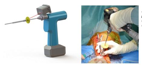
Figure 10.6.1: The AutoGauge prototype as a CAD drawing (left) and in action during a sheep surgery.
