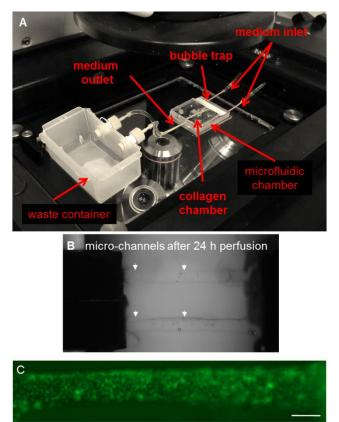
Figure 10.7.7: *Micro-fluidic platform. A.* Set-up of the new microfluidic chamber installed on EVOS® FL Auto Cell Imaging System. **B.** Stable channels embedded in a collagen gel generated in the new chamber. **C.** GFP-labeled HUVEC could be successfully injected in the chamber and were homogenously distributed. Scale bar 100 µm.
