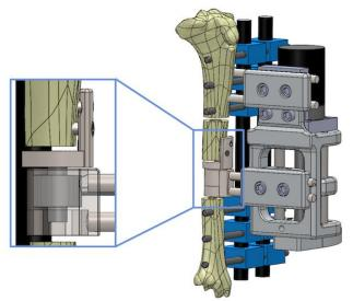
Figure 10.3.2: Illustration of the actuator-driven external fixator with incorporated load cell in the critical size defect (enlarged section).
