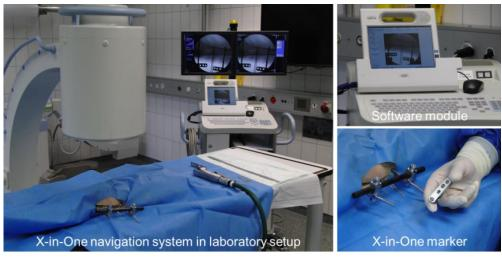
Figure 10.5.3: Navigation tool for assisting rotational osteotomies in a laboratory setup, containing the software module implemented on a tablet computer (upper right) and the special designed markers (lower right).
