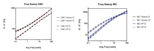
Figure 10.7.3: Viscoelastic spectrum before (black lines) and after (red or blue lines) high hydrostatic pressure treatment. Left panel: CarboxyMethyl Cellulose (CMC); Viscoelastic shear moduli were unchanged upon treatment. Right panel: Methyl Cellulose (MC); Viscoelastic shear moduli displayed a slight loss upon treatment. Steam sterilisation (not shown) would bring to a considerable decrease of viscoelastic moduli.
