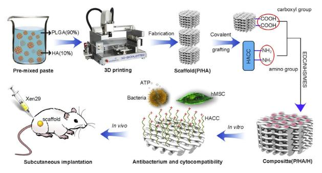
Figure 10.7.2: Schematic illustration for the synthesis and antibacterial mechanism of P/HA/H composite scaffolds (reproduced from Yang et al. Acta Biomater 2016;46:112-28).
