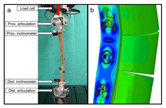
Figure 10.4.1: Test setup with a specimen mounted for mechanical testing (left, a). Principal strains at a hybrid LCP PCA plate as predicted by the Finite Element Analysis (right, b).
