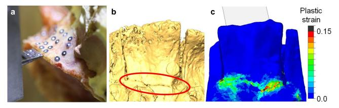
Figure 10.7.1: Experimental test setup (a), induced fracture line (b, red ellipse) and FE-based plastic strains (c).
