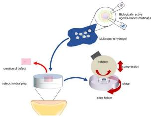
Figure 10.7.9: Experimental set-up for ex-vivo testing of nanocarrier systems.
