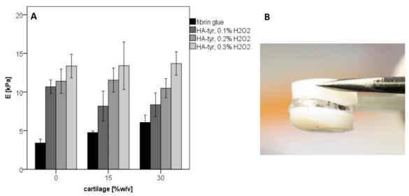
Figure 10.6.5: Compressive modulus of gels loaded with 0, 15 and 30% of cartilage particles. B: HA-tyr mediates the adhesion of two cartilage cylinders to each other from Cavali et al. 2015, ORS abstract.
