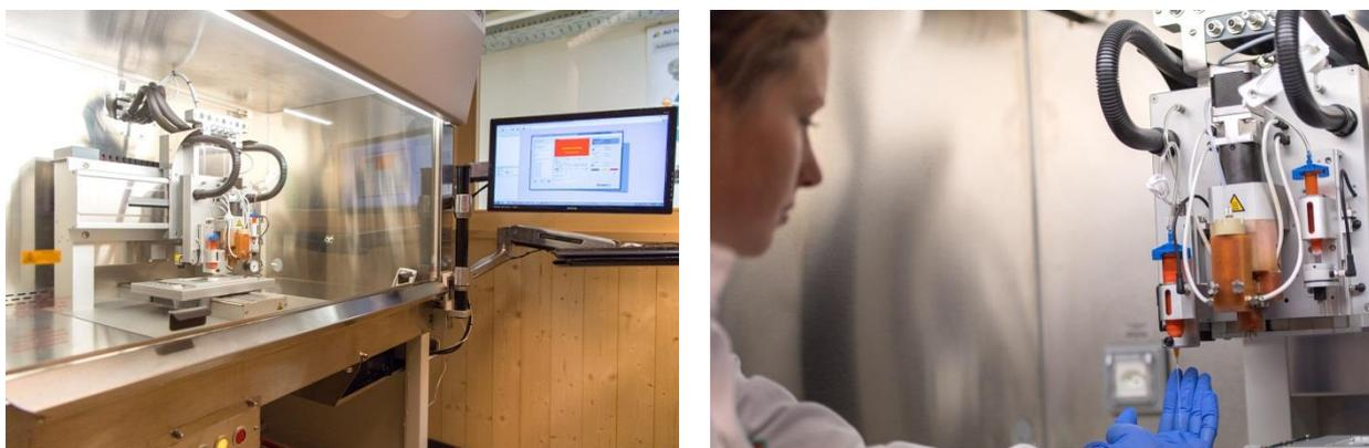
Figure 7.1: AO Research Institute Davos biofabrication unit equipped with state of the art 3D discovery® bioprinter from RegenHU Ltd.
