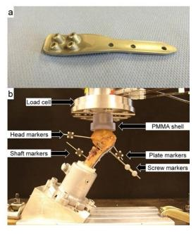
Figure 10.3.4: The new plate prototype for proximal humerus fracture fixation with four short barrels for gliding of its proximal screws (a, top); Test setup with a plated humerus specimen, equipped with retro-reflective markers for optical motion tracking and mounted for biomechanical testing (b, bottom).
