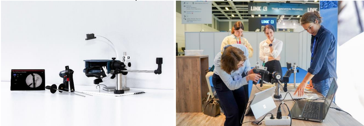
Figure 11.8.1: Final DEHST product (left) and new module for pinning distal radius fractures in practical use at DKOU (right).
